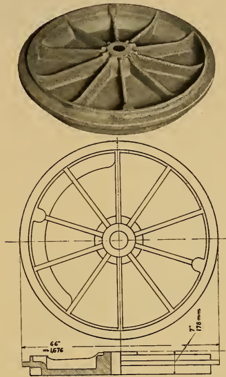
Fig. 15. Marine Engine Cylinder Head—Weight 2400 pounds.
